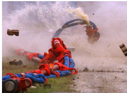
Testing validated SPM® FSR's ability to reduce the danger area around high pressure hydraulic fracturing operations.
