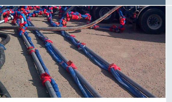
The destructive force of an unrestrained flow line rupture, regardless of the cause, can be devastating and catastrophic to both people and equipment. The SPM® Flow Line Safety Restraint (FSR) system is one of the industry's most utilized restraint systems designed to reduce the area of danger around high-pressure flow line disengagements. Operators and service companies have relied on the SPM® FSR system to enhance safety during pumping operations.
