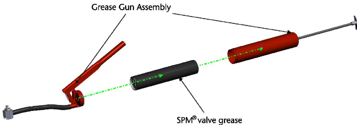
3. Slide the grease gun fitting over the valve's grease fitting.
