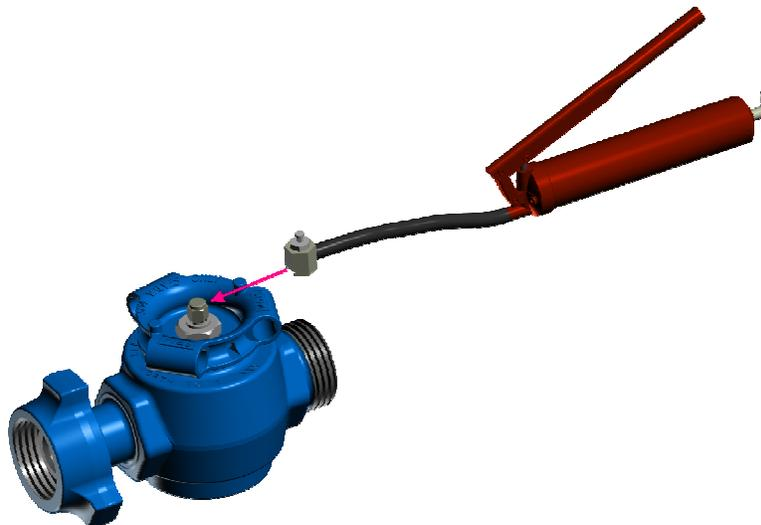
4. Using the grease gun, pump the lever in order to push the grease into the valve. Val-Tex 972 (SPM<sup>®</sup> Part Number P32553) stick grease is recommended.
