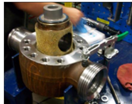
10. Install body cap seal (7) and back-up ring (6), where required, onto body cap (5) with valve assembly grease.
