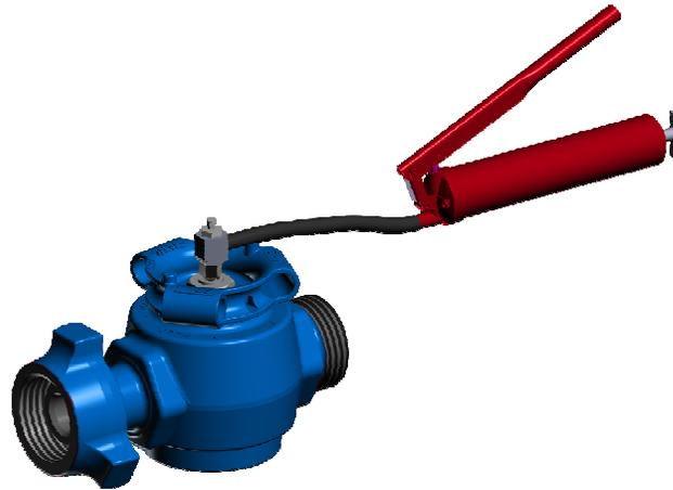
5. Keep pumping the grease gun until you can see the grease expanding around the plug. Inject a minimum of 6,000 psi to insure proper filling of valve. (gauge reading on pneumatic grease gun)
