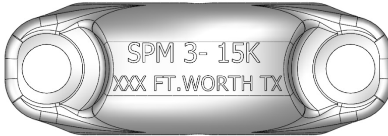
Top View – Non Threaded Safety Iron ® Half (Showing identification markings)
